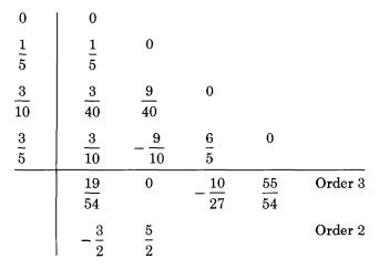
Similar arguments to those used for the first-order solution can now be applied. Since the order 3 solution is acceptable, while the order 4 solution is not, we anticipate possible trouble in the range  $[x_n + 3h/5, x_n + h]$ . As a result, it is only safe to integrate forward a distance 3h/5 during the current step. We therefore seek a third-order formula of the form
